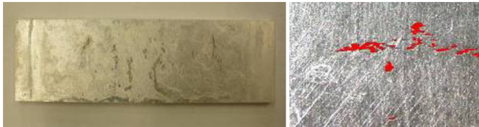
Fig. 5 Image analysis of a corroded surface
