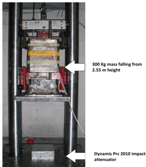
The resulting deceleration on the 300 Kg mass have been plotted on matlab.
