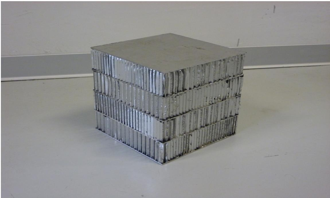
Since the supplier couldn't provide us the compressive yield stress, we managed to verify the typical mechanical behavior of honeycomb panels and the compressive yield stress by testing our component on a press machine:
