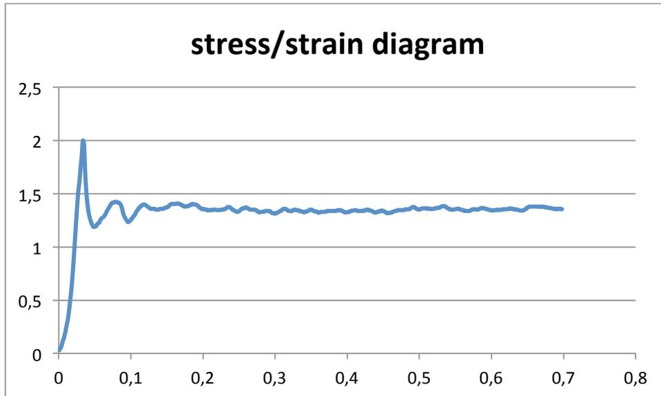
The main features of the diagram are the linear stress-strain elastic behavior and the flat stress-strain plastic behavior; during the plastic behavior, the material shows the typical buckling effects. The elastic behavior is responsible of the peak deceleration of the mass at the beginning of compression of any honeycomb layer: in order to start the buckling behavior, the force given by the mass to the component reaches the value able to yield the honeycomb.
